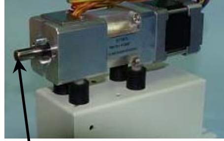
Remove dust off the plunger.
